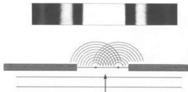
Fig.5: Schematic of Fresnel's work (1815) [10]
