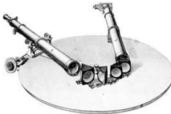
Fig.11: The spectroscope of Kirchoff [16]
