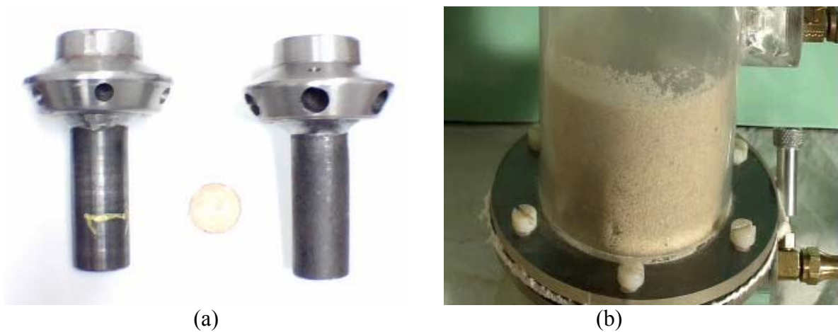
Fig. 2: (a) Two of the eight nozzles that were simulated. (b) The laboratory test bench.
