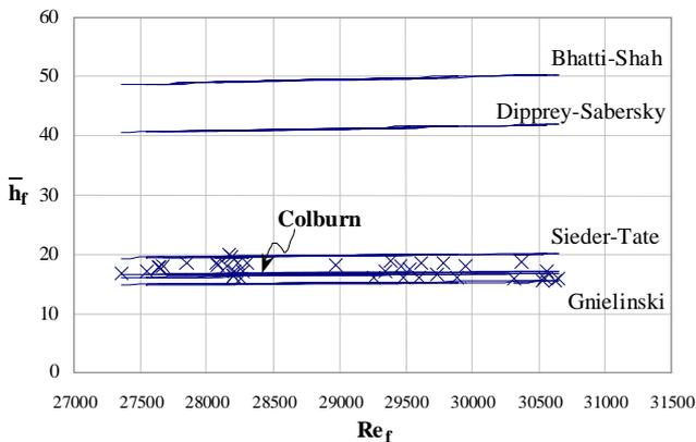
Figure 3. Experimental ("x") vs predicted (continuous lines) heat transfer coefficients.
