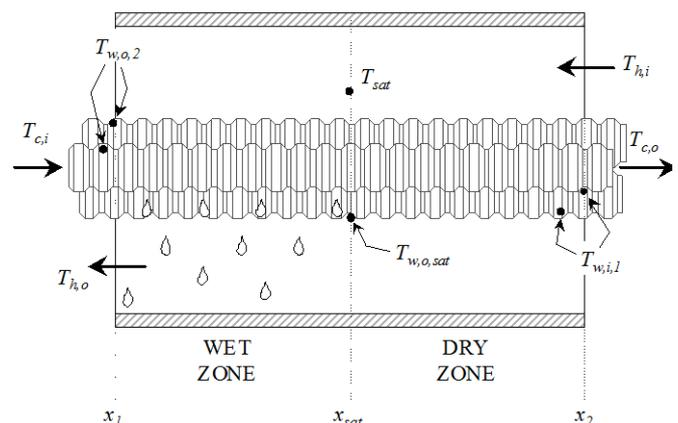
Figure 1. Thermal configuration of the prototypes.
