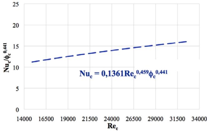
Figure 4. Experimental data correlation as a relative humidity function.
