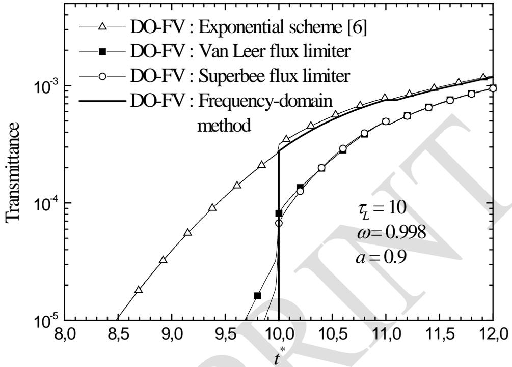
Figure 3: Temporal distribution of hemispherical transmittance; comparison between the Van Leer flux limiter, the Superbee flux limiter, the exponential interpolation scheme [6], and the frequency-domain method at early time periods.
