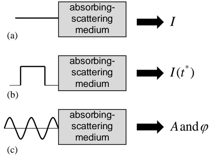
Figure 6: Schematic representation of optical tomography techniques: (a) traditional steady-state; (b) time-dependent; (c) frequency-based.
