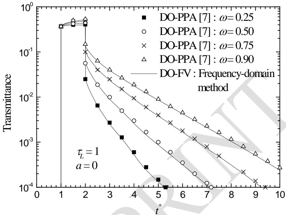
Figure 4: Temporal distribution of hemispherical transmittance; comparison between the frequency-domain approach and the DO-PPA method [7].
