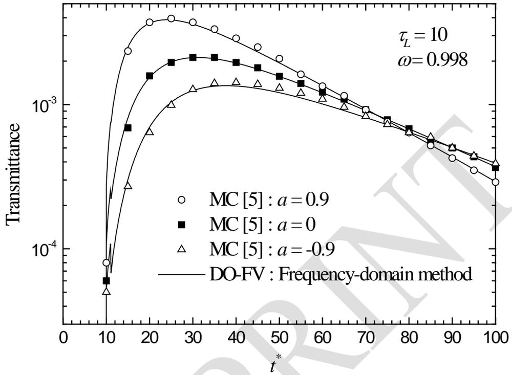
Figure 2: Temporal distribution of the hemispherical transmittance; comparison between the frequency-domain approach and a Monte Carlo formulation [5].
