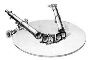
Fig.11: The spectroscope of Kirchoff [16]
