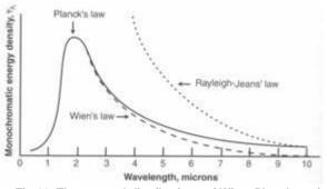
Fig.11: The spectral distributions of Wien, Planck, and Rayleigh-Jeans [18]
